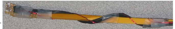
Figure 3: A calibration wand consisting of a Knowles micro-speaker and an LED collocated at the end of a pencil was used to obtain the fundamental matrix.
