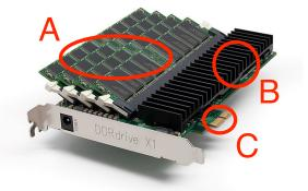
ANSWER: There are RAM chips (A) attached to the main board. The heatsink (B) radiates off excess heat from the main board, which connects to the rest of the computer through the connector (C).
