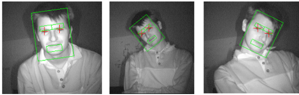
Figure 6: Face feature detection based on eye location when the head is in different orientation
