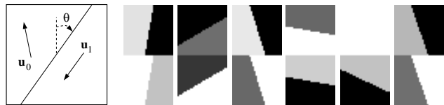
Figure 1: Discontinuity training set. Left: model for generating synthetic flow fields. Right: samples from the training set. The horizontal component is shown above the vertical component. Black denotes pixels moving left or up or u and v respectively. White denotes motion right or down.
