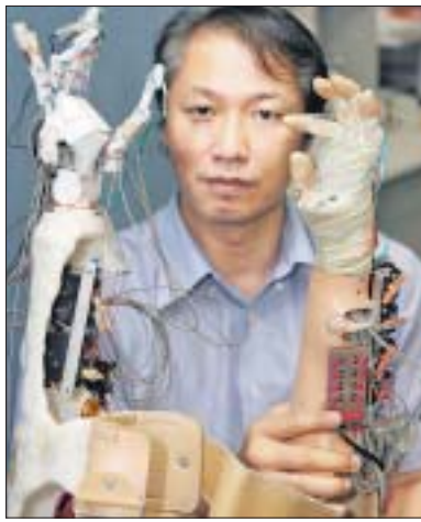
■ Tokyo University Associate Professor Hiroshi Yokoi displays a robot hand which is able to grip a raw egg and crush an aluminium can. The artificial hand has myoelectrical sensors to measure surface Electromyography (EMG) on the elbow of amputee, to estimate the motion to control the movement of fingers —AFP
