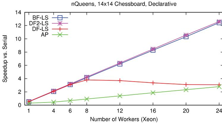
Fig. 8. Performance scaling of schedulers on Xeon (nQueens).
