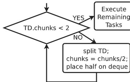
Fig. 2. Processing a task descriptor with auto-partitioner.
