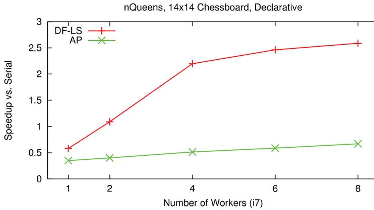
Fig. 4. Performance scaling of schedulers on i7 (nQueens).
