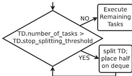
Fig. 1. Processing a task descriptor with simple partitioner.
