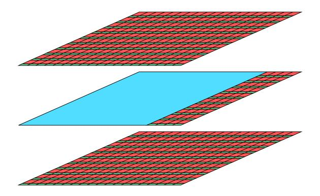
Red blocks - TCU clusters. Green blocks - memory modules. Blue block - the ICN. <u>Main points of this slide</u>: ICN is confined to one layer. It is a middle layer. Can share with other functions. Memory ports in external layer.
