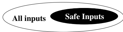
Figure 1. An input validation vulnerability occurs when the set of all inputs for P (in white) is a superset of the set of safe inputs for P (in black). The set difference is the set of exploits for P .
