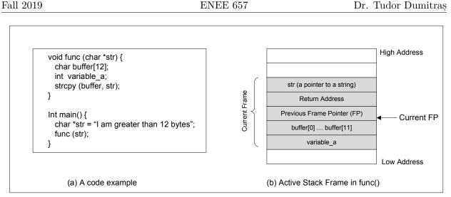
Finding the offset R of the memory location that stores the return address. If the source code for a program like stack is available, it is easy to guess R accurately, as illustrated in the previous figure. Another way to get R is to run the executable in a (non-root) debugger.
