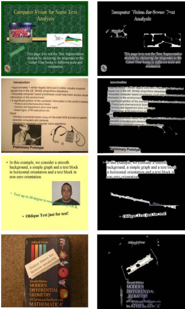
Fig. 7a–d. In this example, we test the power of the text-segmentation algorithm for different presentation/poster and outdoor scene text layout. Top-to-bottom images are a–d . a,c Presentation slides with different text size and orientation, different graphs, and complex or simple background. c Image of a poster with simple background. d Image of a book on textured background. The results of text segmentation are shown in the second column
