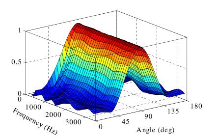
• By weighting/filtering and summing signals from different microphones, a `virtual' directivity pattern may be produced
