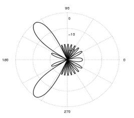
• Sensor-dependent filters implement frequency-dependent complex weights to obtain a desired response over the whole frequency/angle range of interest
