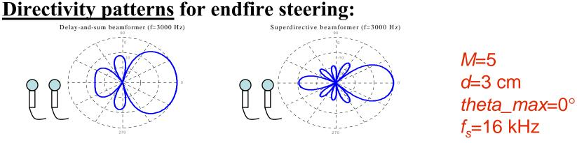
Superdirective beamformer has <u>highest DI</u>, but very <u>poor WNG</u> hence problems with *robustness* (e.g. sensor noise) !
