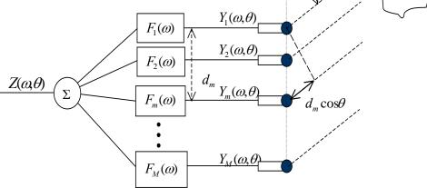
• Hence `spatial filter design' based on microphone characteristics + microphone array configuration.
