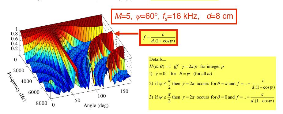
• Beamwidth: for a uniform delay-and-sum beamformer
