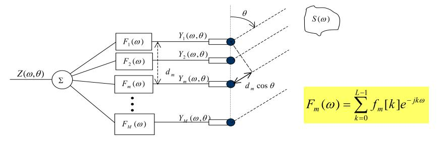
Terminology: `Broadside' direction:  $\theta = 90^{\circ}$  `End-fire' direction:  $\theta = 0^{\circ}$
