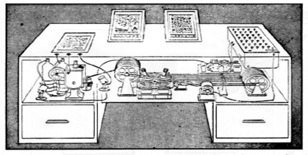
Memex in the form of a desk would instantly bring files and material on any subject to the operator's fingertips. Slanting translucent viewing screens magnify supermicrofilm filed by code numbers. At left is a mechanism which automatically photographs longhand notes, pictures and letters, then files them in the desk for future reference (*LIFE 19*(11), p. 123).
