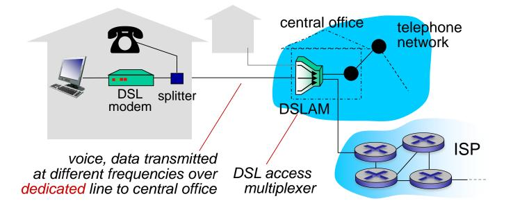
use existing telephone line to central office DSL access multiplexer
