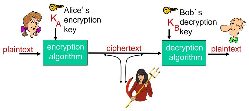
m plaintext message  $K_A(m)$  ciphertext, encrypted with key  $K_A(m) = K_B(K_A(m))$
