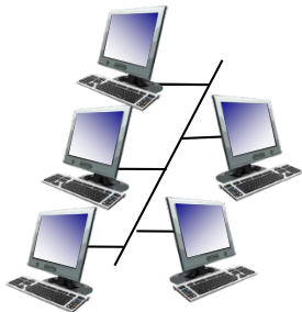
shared wire (e.g., cabled Ethernet)
