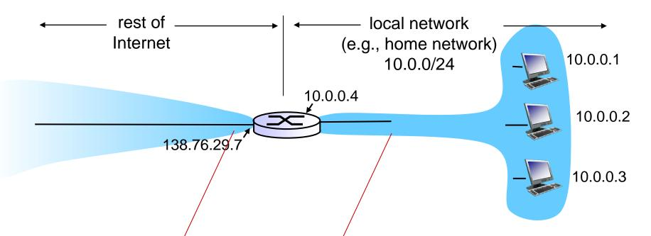
all datagrams leaving local network have same single source NAT IP address: 138.76.29.7,different source port numbers datagrams with source or destination in this network have 10.0.0/24 address for source, destination (as usual)
