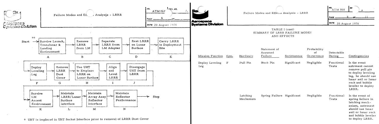
\*\* The loss of corners due to environmental stress during transportation to the lunar surface would result in a linear degradation of the return signal to earth. A design safety factor has been included in the Array to preclude the probability of corners fracturing due to
