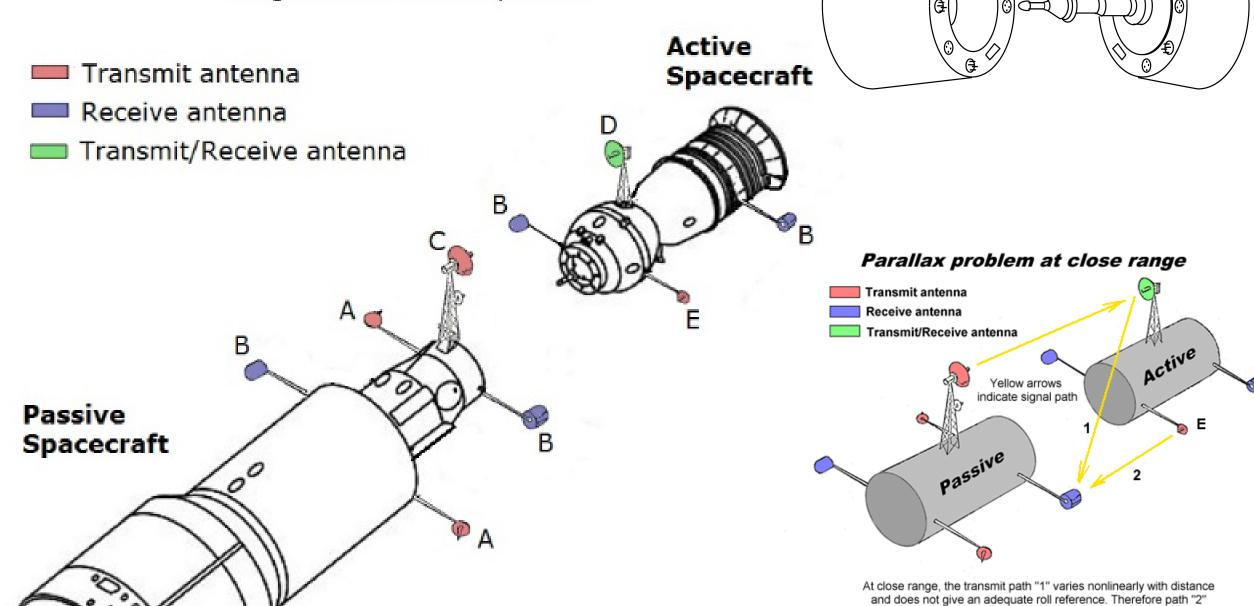
using antenna "E" is used at very close range.
