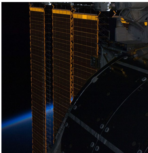
Figure 4: ISS "Blanket" Solar Panel Arrays- The large solar arrays are the main source of power on the ISS.
