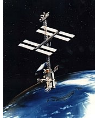
Figure 1: Space Station Freedom Concept Design - This design was optimized for gravitational gradient stability, as seen by its large height compared to its other dimensions.
