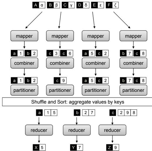
**Figure 1: Illustration of MapReduce: mappers are applied to input records, which generate intermediate results that are aggregated by reducers. Local aggregation is accomplished by combiners, and partitioners determine to which reducer intermediate data are shuffled.**
