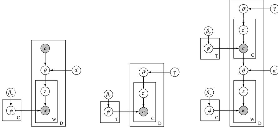
Figure 1: Graphical Models for three topic modeling approaches: Topic model using words only (left), A topic model using tags only (middle), and a model using both tags and words (right).
