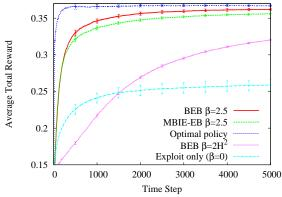
Figure 2. Performance versus time for different algorithms on the chain domain, averaged over 500 trials and shown with 95% confidence intervals.
