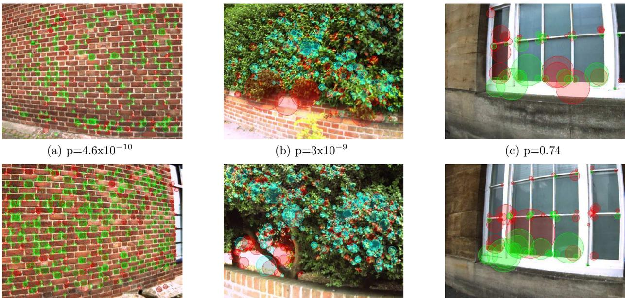
Figure 3. Some similar-looking images from different parts of the workspace correctly assigned low probability of having come from the same place. Words common to both images are shown in green (in blue for (b)), others in red.
