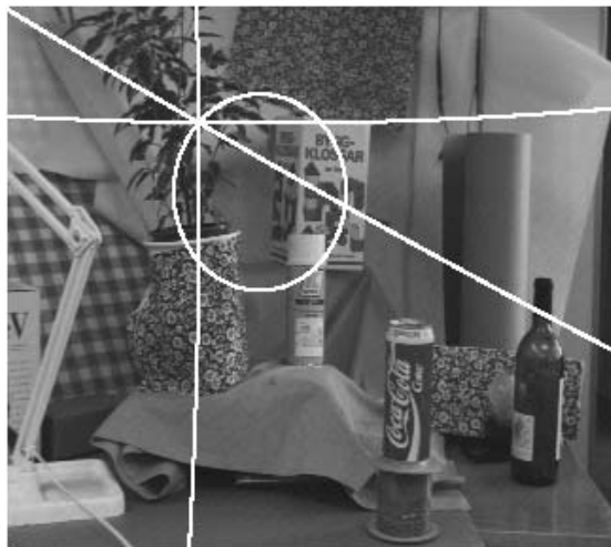
Figure 5.20: KTH scene: Curves separating the translational components of the \alpha -, \beta -, \gamma -vectors and coaxis vectors (\alpha, \beta, 0) . At their intersection lies the FOE.
