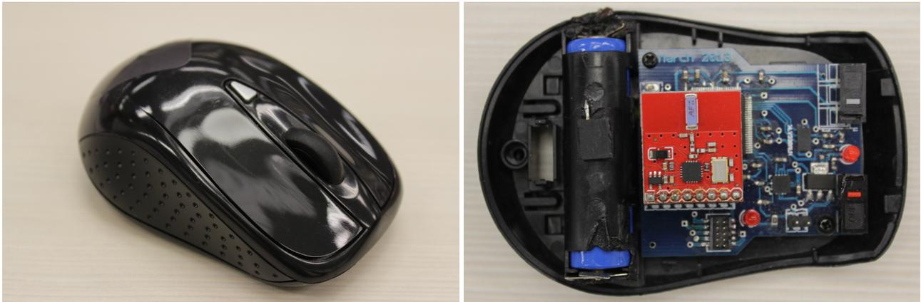
Figure 9: Wireless MEMS Mushaca with accelerometer and gyroscope supporting a standard USB optical mouse interface.
