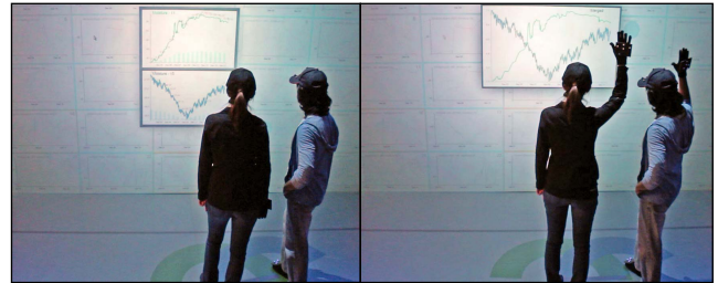
Figure 4: A hybrid merge interaction that uses proxemics to stack the lenses when the users are close (left) and changes the merge mode to content overlay when they perform a collaborative gesture (right).
