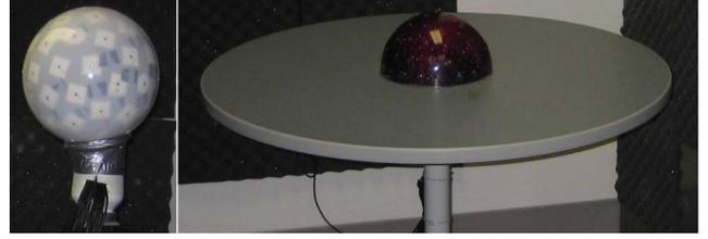
Fig. 1. Spherical (left) and hemispherical (right) microphone arrays.
